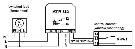
The normally closed contact MKW 1 is used to control an extractor hood (OPEN window > magnetic contact closed > fume hood in operation)
