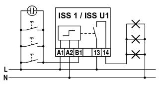
After applying the supply voltage to A1 and A2, the switching state can be changed permanently by a push pulse to B1.
